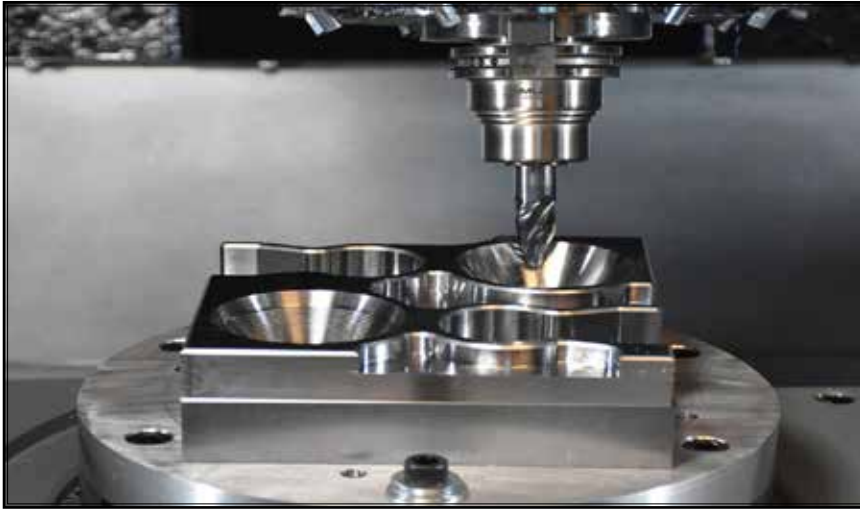
Gambar 6.1 Toolpath surface Roughing dan finishing
